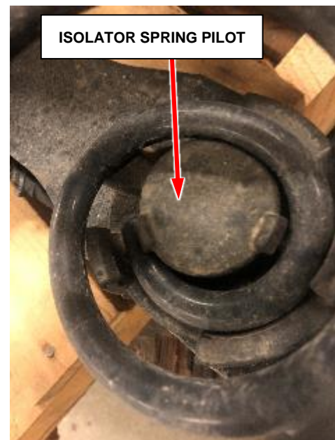
Figure 2 – Coil NOT On Top of the Isolator Spring Pilot
