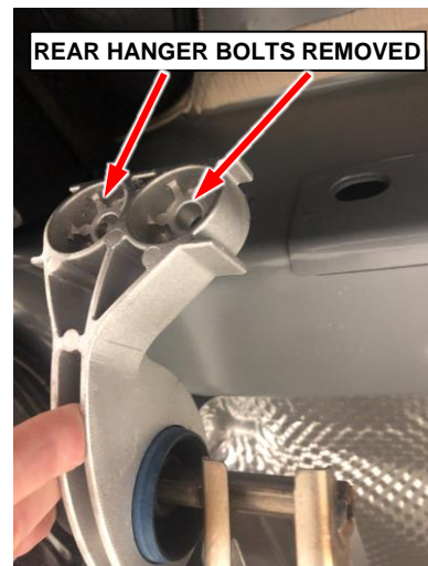
Figure 5 – Rear Exhaust Hangers
