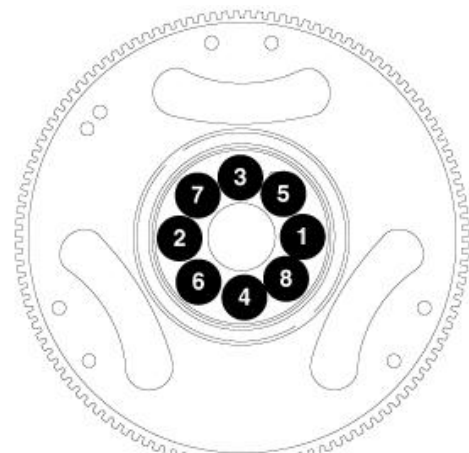
Figure 29 – Flexplate Tightening Sequence
