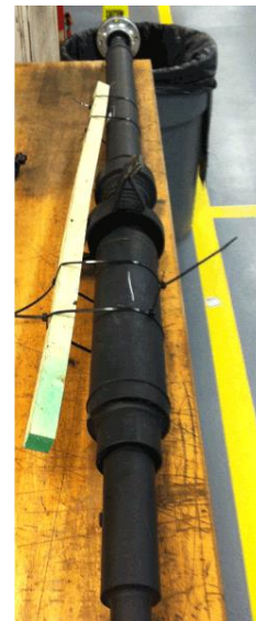
Figure 11 – Supporting Propeller Shaft
