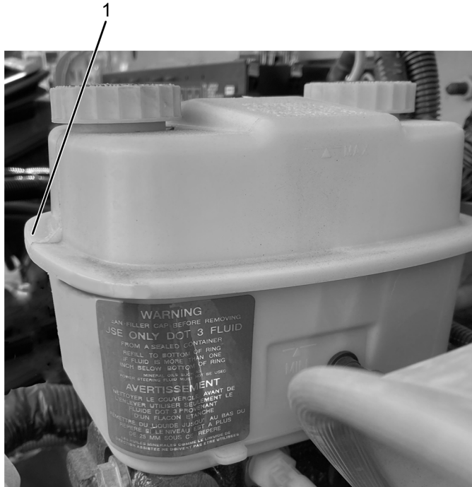
Figure 7. Brake Fluid Reservoir – Fluid Mid-Level Measurement 1. Reservoir ring
