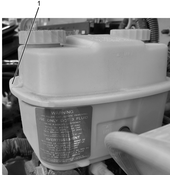
Figure 20. Brake Fluid Reservoir – Fluid Mid-Level Measurement
