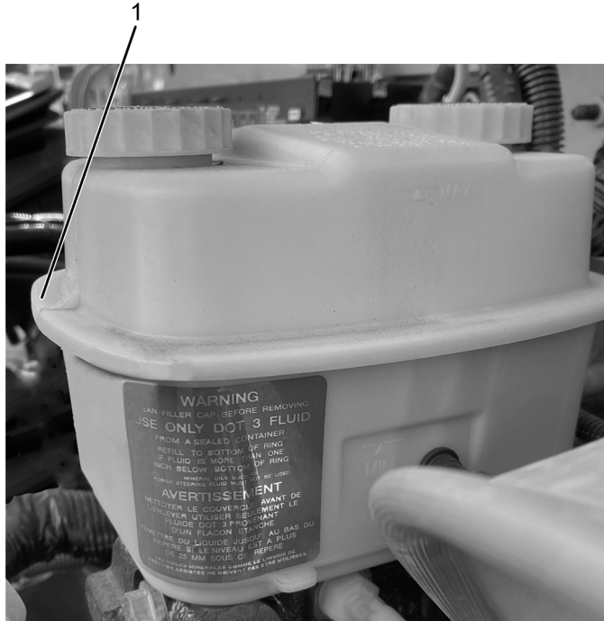
Figure 11. Brake Fluid Reservoir – Fluid Mid-Level Measurement
