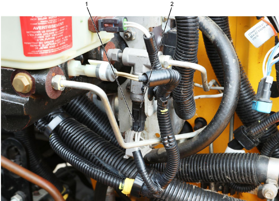
Figure 1. Brake Pressure Switch Connector Location
