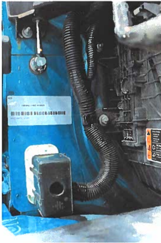
Figure 23. 1703F Bulkhead Connector with Jumper Harness Installed
