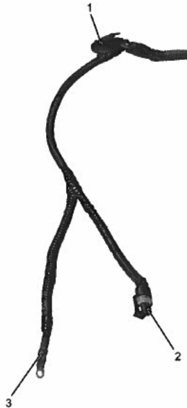
Figure 25. Modified Low Fluid Switch Connector, Hydro-Max Brake Pressure Terminal and 5 Amp Fuse from IP Cowl Harness (Ground and Low Level Sensor Harness)
