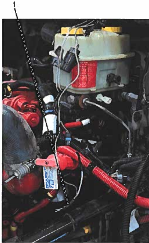
Figure 41. Circuit A090F with Heat Shrink
