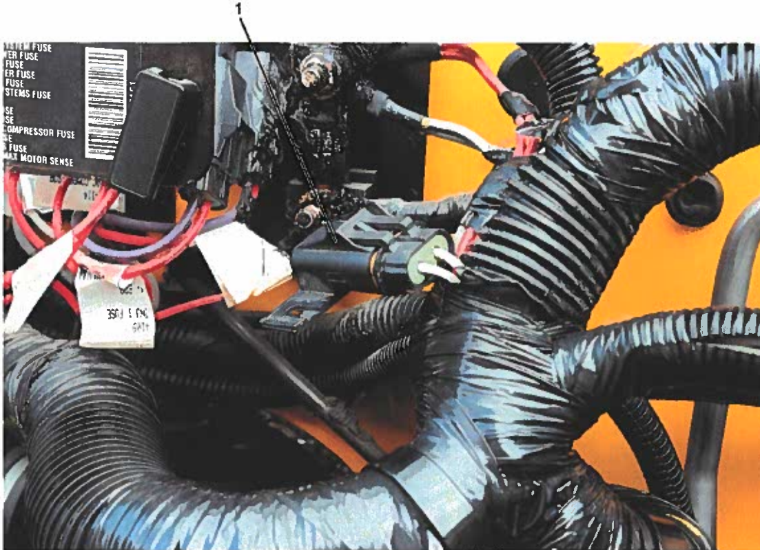
Figure 6. 5 Amp Fuse and Cover
