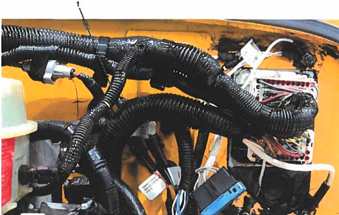
Figure 15. New Low Level Sensor Connector Routing
