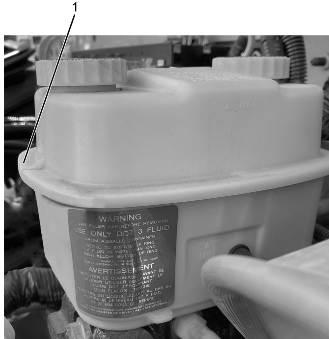
Figure 7. Brake Fluid Reservoir – Fluid Mid-Level Measurement
