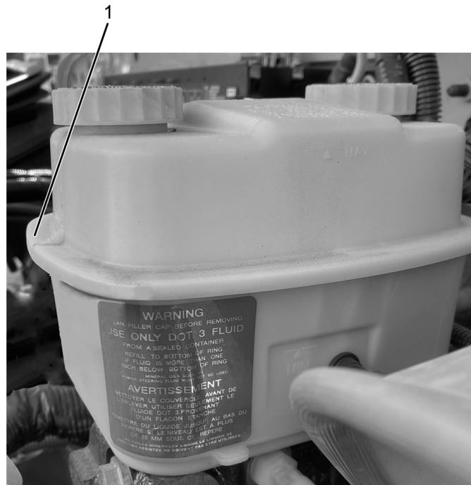
Figure 12. Brake Fluid Reservoir – Fluid Mid-Level Measurement
