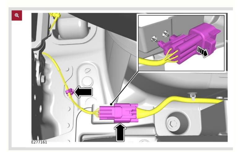
**6.** Inspect both rear lamp assembly wiring harnesses for damage.
