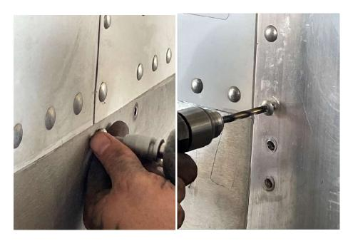
4. Remove the nutted floor screws attaching the front of the floor boards to the rear of the coupler assembly. Continue by removing the baserail bolts from both sides of the rail that are attaching the coupler assembly to the trailer walls.
