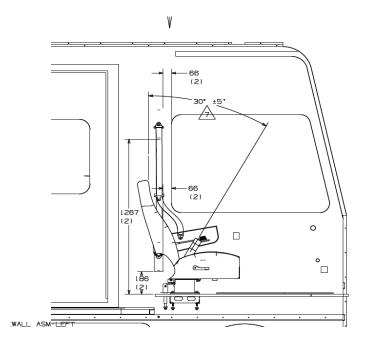
3. Torque bolt under each cap to 45+/-3.5 Nm (33+/-3 ft-lb)
