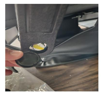
2. Ensure 30-degree angle for each seat belt buckle is met. Loosen bolt under cap and correct angle if required.
