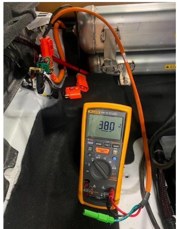
Figure 12 – PHEV Circuit Testing
