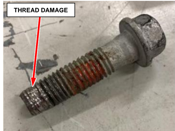
Figure 21 – Inspect Bolt Threads
