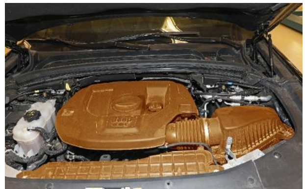
Figure 20 – Engine Cover and Air Cleaner Housing Assembly
