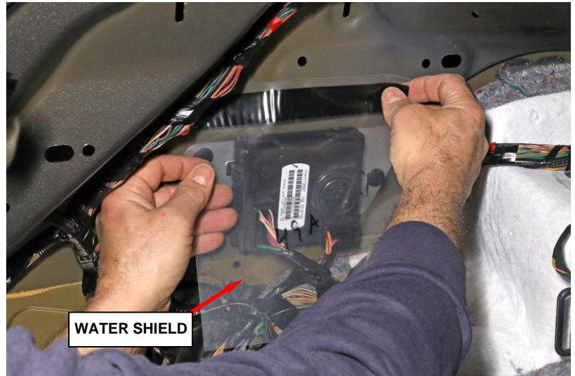
Figure 28 – Install Water Shield
