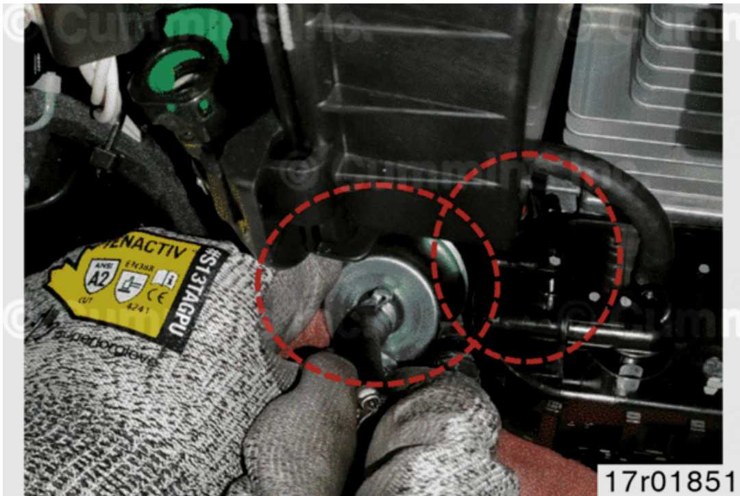
Figure 12, Pull/disconnect inlet hose
