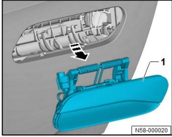
Disconnect the connector <1> from the door handle assembly.
