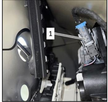
• Once the locking plate <1> is in the unlocked position (as shown), the pins <arrows> on the door handle will be released.
