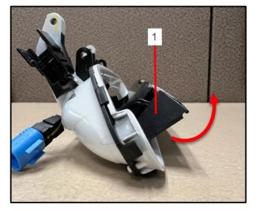
• Once the tabs <1> have been released, rotate the lamp out of the retaining tab <2> in the direction indicated <arrow>.
