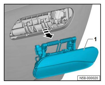
• Pivot out the door handle assembly <1> in the direction of <arrow> and remove.
