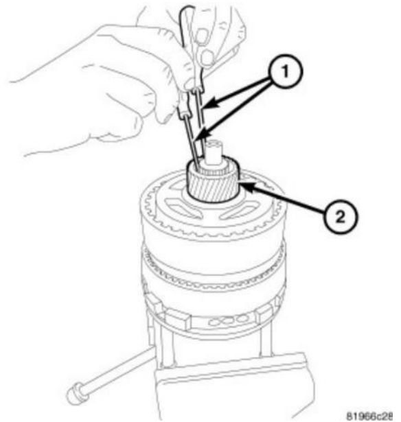
Figure 32 – Sun Gear Retaining Clip
