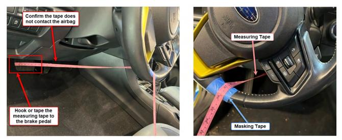
**STEP 4:** Write a reference mark on the taped section of the steering wheel. Make a measurement to the brake pedal in its current position and record it.
