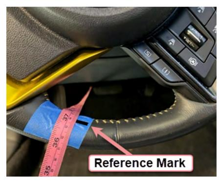
**STEP 5:** Press the brake pedal until the stop lights come on (a second person or the SSM4 with the stop lamp switch PID selected) then measure again to determine the extension of the switch.
