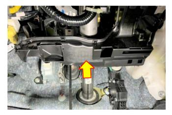
**STEP 2:** Using a feeler gauge, check the switch plunger extension length between the stop lamp switch threads and the stopper section of the brake pedal.
