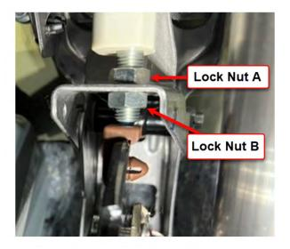
**IMPORTANT:** Never adjust the pedal stroke to less than 3mm. Doing so may cause the stop lamp to illuminate without pressing the brake pedal.
