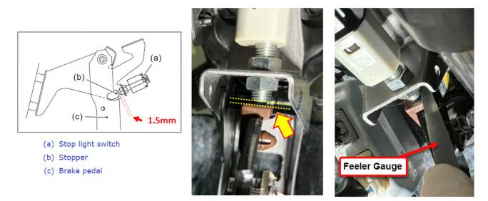
The plunger portion of the switch should extend between the stopper section of the brake pedal and the stop lamp switch threads 1.5mm (0.06 in) in length.
