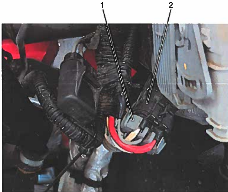
Figure 5. Booster Pump Motor Jumper Harness Connector
