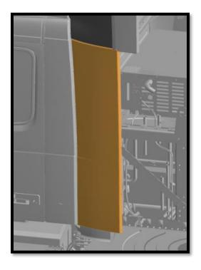
Step 4. Reposition the lower ESS's. Install the ESS mounting fasteners.
