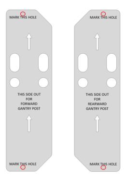
Step 13. Drill a 14mm hole at all four marked locations. Paint the drilled holes for corrosion protection.
