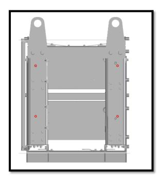
Step 14. Remove the bottom screw on both the inlet and outlet coolant ports on both gantry mounted ESS's to allow borescope access.
