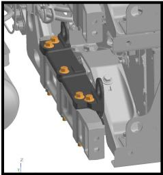
Step 6. Carefully slide both lower ESS outward so the inboard screw can be accessed with the borescope.
