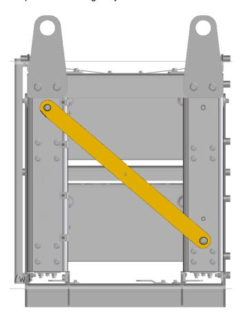
Step 11. Place drilling template on gantry posts according to instructions on the template.
