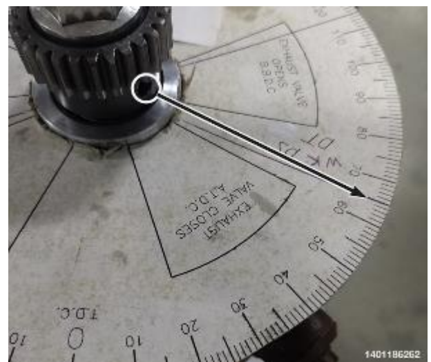
Figure 194 – Installing a Printed Paper Degree Wheel from the Internet
