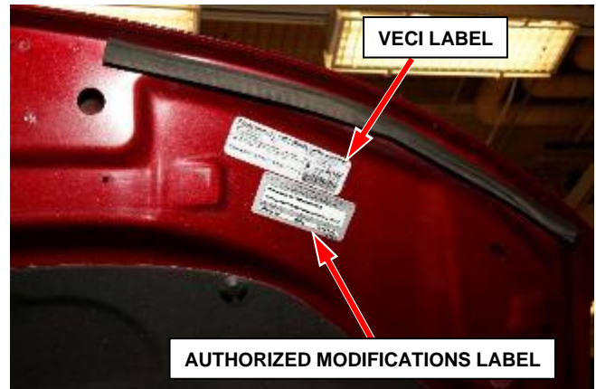
Figure 204 – Apply Authorized Modifications Label Near VECI Label (Specific Vehicle May Look Different)
