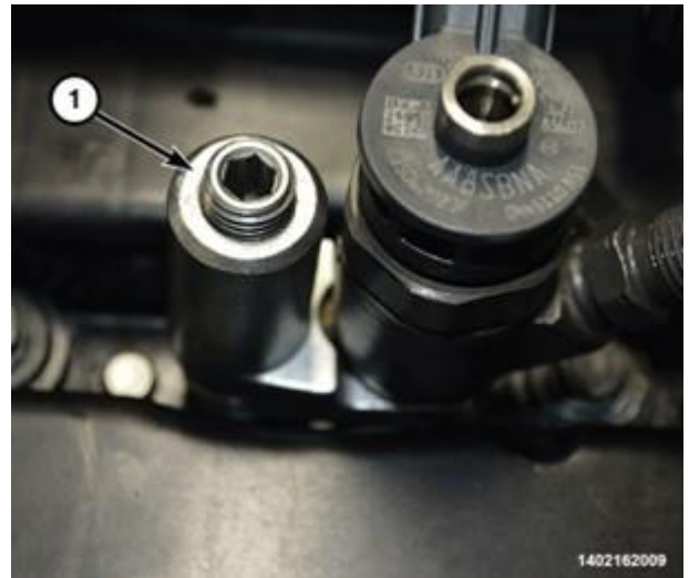
Figure 134 – Remover, Fuel Injector VM.10358A
