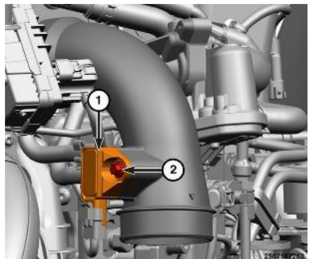
Figure 27 – Differential Pressure Sensor
