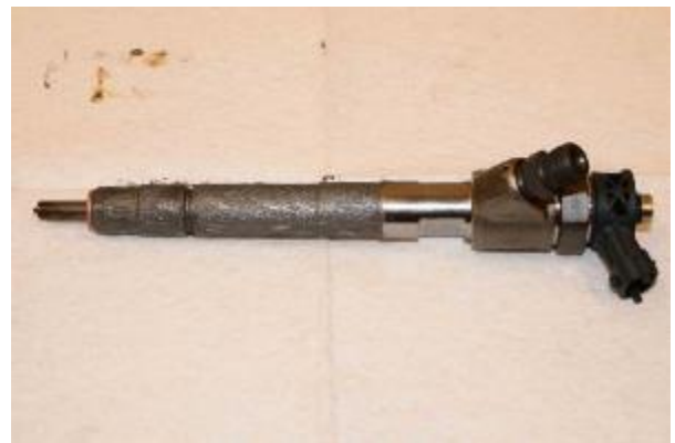
Figure 142 – Lubricate the Fuel Injector
