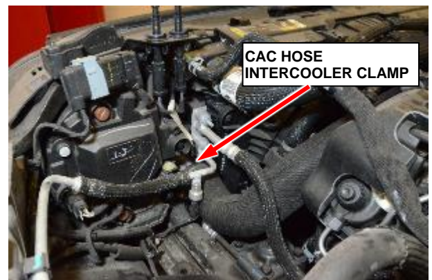
Figure 96 – CAC Hose from Intercooler
