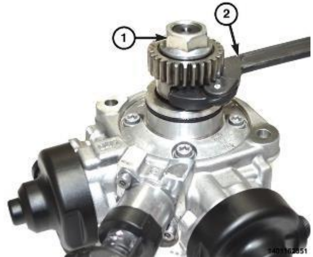
Figure 170 – Installing the Drive Gear on the HPFP
