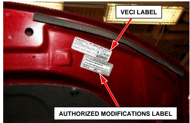
Figure 199 – Apply Authorized Modifications Label Near VECI Label (Specific Vehicle May Look Different)
