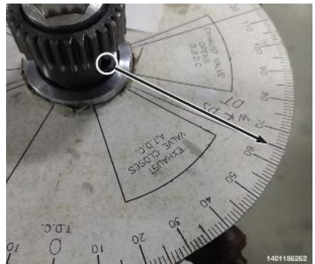
Figure 194 – Installing a Printed Paper Degree Wheel from the Internet
