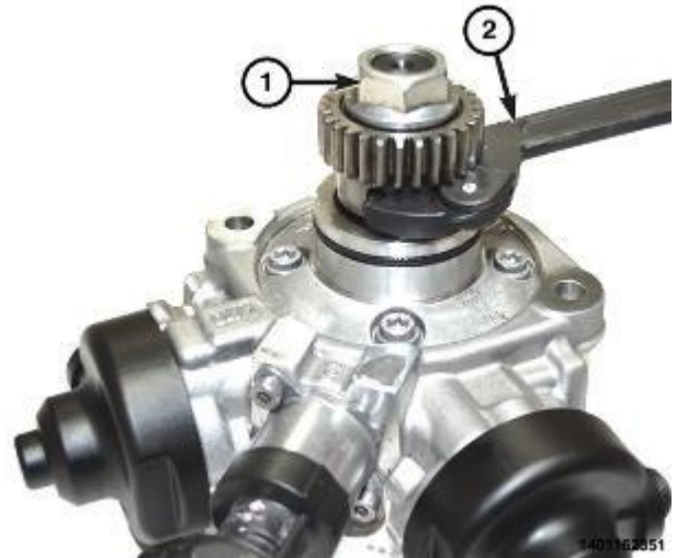
Figure 170 – Installing the Drive Gear on the HPFP
