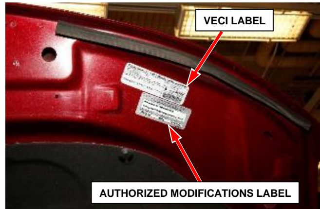
Figure 147 – Apply Authorized Modifications Label Near VECI Label (Specific Vehicle May Look Different)
