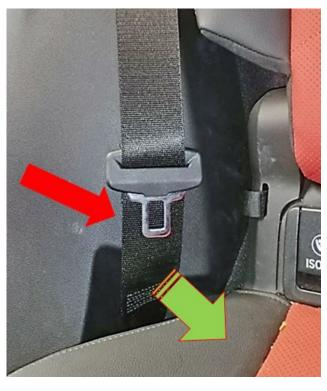
If the belts are not mounted correctly, grasp the lower part of the belt webbing (red arrow) below the latch and pull the belt firmly in the direction of the green arrow (toward center of vehicle) to release the pinched belt (the right rear passenger seat is shown).
