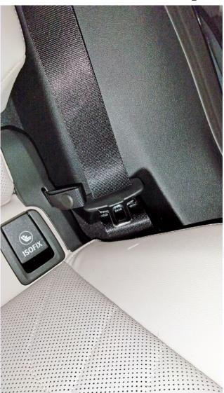
The safety belt webbing is slightly clamped by/pinched under the C-pillar trim at the bottom. The latch is held in a low position. NOT OK
