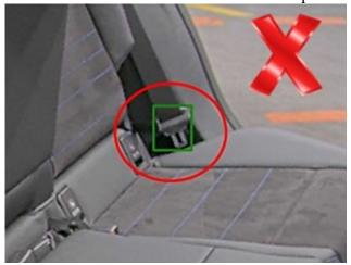
The safety belt webbing is slightly clamped by the C-pillar trim at the bottom. The latch is held in a low position. NOT OK
