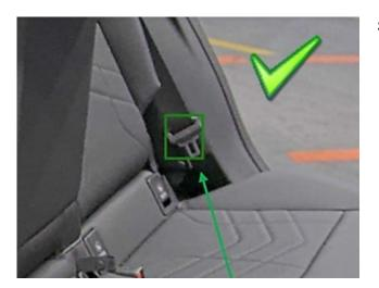
Safety belt installed correctly. OK
