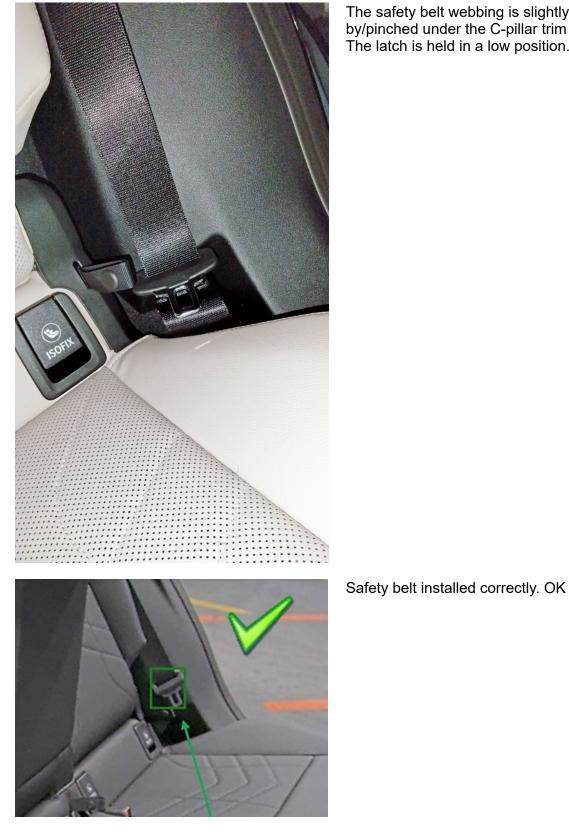
The safety belt webbing is slightly clamped by/pinched under the C-pillar trim at the bottom. The latch is held in a low position. NOT OK
