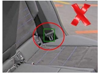
The safety belt webbing is slightly clamped by the C-pillar trim at the bottom. The latch is held in a low position. NOT OK 72 02 23\_RECALL 23V-260: SAFETY BELT REAR SEAT (LEFT AND RIGHT)
