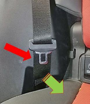
If the belts are not mounted correctly, grasp the lower part of the belt webbing (red arrow) below the latch and pull the belt firmly in the direction of the green arrow (toward center of vehicle) to release the pinched belt (the right rear passenger seat is shown).
