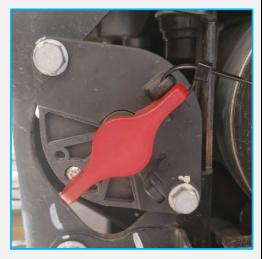
2. Locate the PVM (1) at the rear of the truck, installed above the E-axle.
