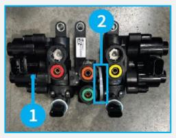
2. Locate the label (2) and record the serial number from the new PVM (1).
