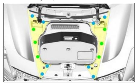
4. Partially remove the indicated gasket (luggage compartment weatherstrip).
