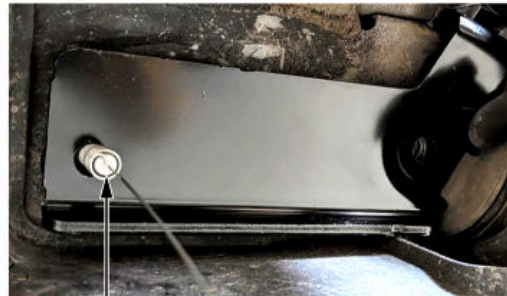
Bolt guide wire and bolt will be seen here.
