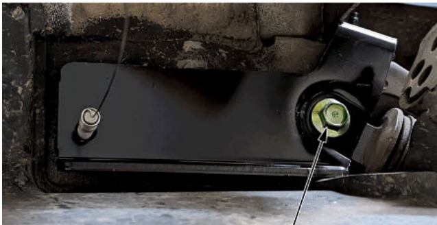
REAR TRAILING ARM FRONT MOUNTING BOLT Do not torque to specification.
