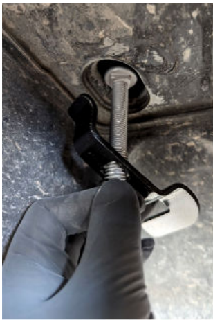
Insert the head of the bolt through the drain hole.
