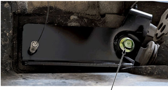
REAR TRAILING ARM BOLT Do not torque to specification.
