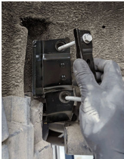
Align bracket with flange facing towards the front of the vehicle, over the two brace studs, then install the two bracket bolts.
