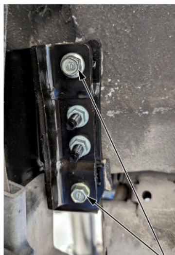
8 mm NUTS 21 N·m (15.5 lb-ft) Tighten.
