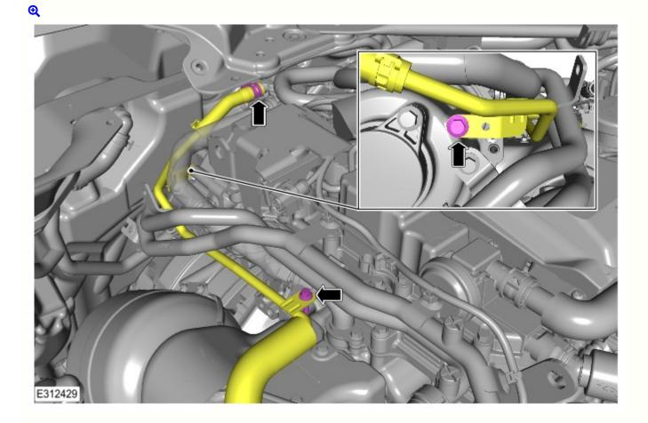
6. Remove and discard the turbocharger coolant inlet pipe.
