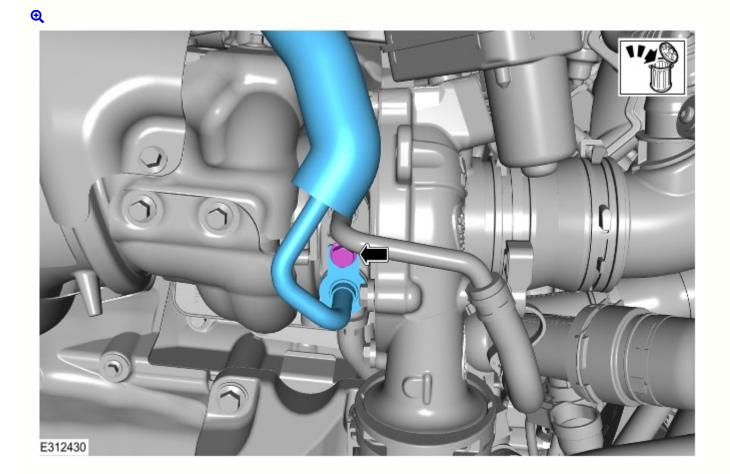
7. Release the turbocharger outlet pipe.
