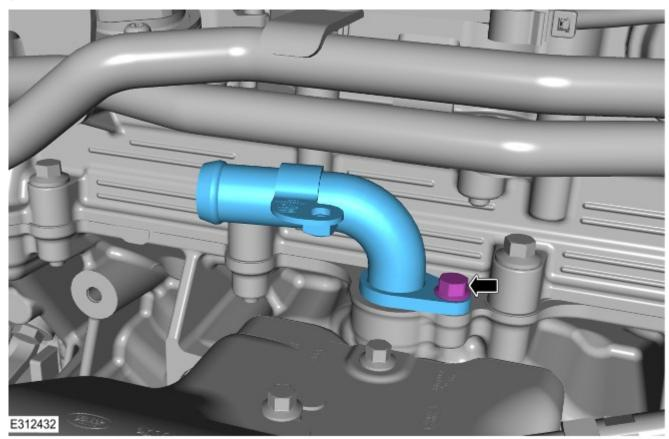
**10.** Install the new engine coolant elbow.
