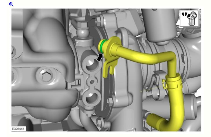
8. Release and reposition the engine coolant hose.
