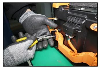
4. Replace the two voltage temperature sensor wire harnesses (VTSWH) with the new parts.
