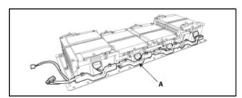
5. <u>During re-assembly</u>, insert the battery temperature sensor into the battery pack lower side area shown.
