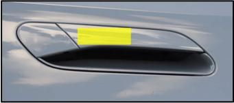
Press firmly in the area shown on the front door handle covers to adhere the foam pad to door handle cover.
