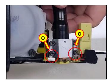
14. Mark all 4 bolts with paint after installing.
