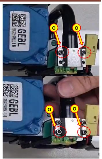
14. After installing, mark all 4 bolts with paint.
