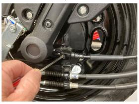
5. Remove the speedometer cable.
