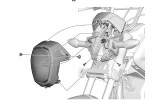
Note: Be careful to pull the lower part of the headlight outward slightly, then release the tab that secures the meter cover to the headlight assembly and pull the assembly straight out.
