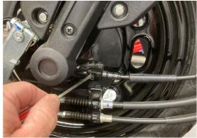
5. Remove the speedometer cable.
