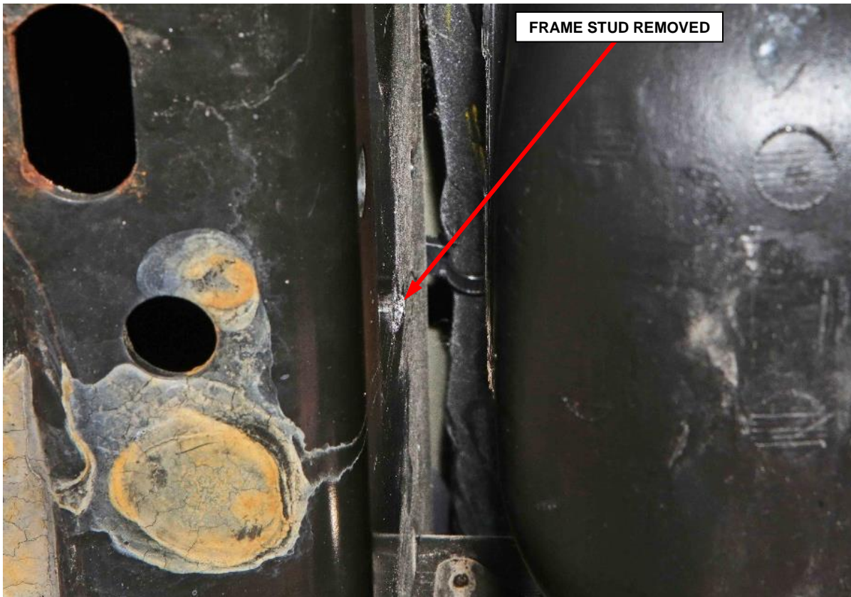
Figure 7 – Frame Stud Removed
