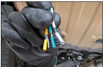
11. Take the new 4-pin wire harness extension, match the corresponding colors and crimp each of the four (4) wires butt-connectors to the vehicle harness.
