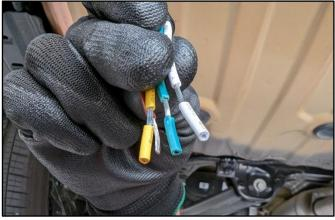
11. Take the new 4-pin wire harness extension, match the corresponding colors and crimp each of the four (4) wires butt-connectors to the vehicle harness.
