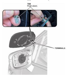
4. For Odyssey driver side mirror only, make sure to install the two long tabs (included in the kit) onto the new mirror.
