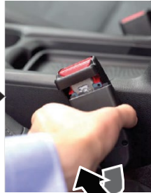
Remove the cover by gently pulling it away and downward.
