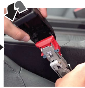
Then remove the upper cover by pulling it away and upward.
