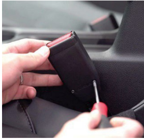
Carefully remove the 2 Torx screws from the cover using a T10 Safety Torx Bit.
