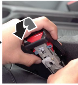
Then remove the upper cover by pulling it away and upward.
