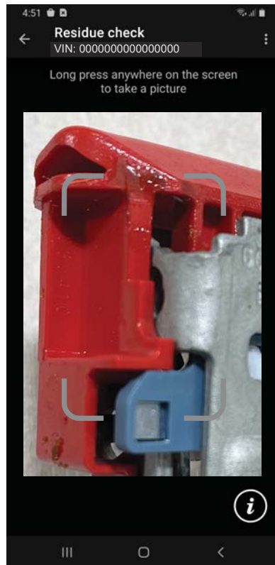
Frame the buckle within the guides, making sure to capture the residue and long-press anywhere on the screen to take the picture.
