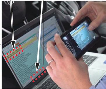
Frame the HDS screen in landscape orientation, making sure to capture the VIN and DTC(s) and long press anywhere on the screen to capture the picture.
