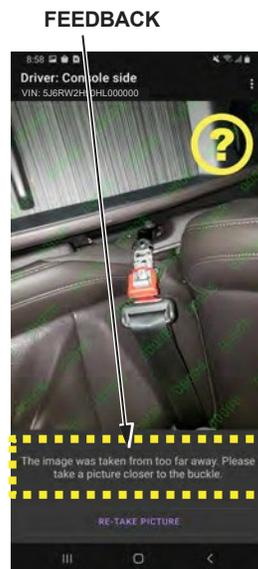
If the application is unable to verify the repair, a "?" or "X" will be displayed in the top right corner of the screen and feedback will be provided on the bottom of the screen to assist in improving the next picture retake.
