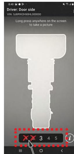
When an "X" is displayed, it will be recorded by the strike counter at the bottom of the screen. If a fifth strike is issued, the application will proceed to the buckle replacement path.
