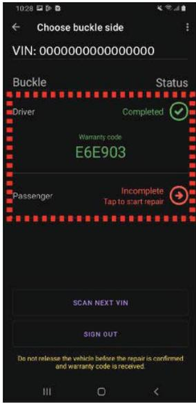
The warranty code for this repair can be retrieved from the buckle status screen at any time by logging into the Buckle Service app using the iN credential of the technician who performed the repair.
