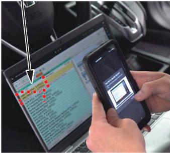
Connect HDS to the vehicle, perform an ALL DTC Check and expand the SRS/SWS DTC Menu to display the SRS DTC(s).
