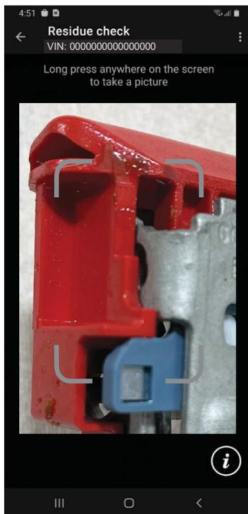
Frame the buckle within the guides, making sure to capture the residue and long press anywhere on the screen to take the picture.
