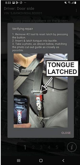
Insert the Seatbelt Tongue into the buckle and confirm it is latched. Pull up on the seatbelt to provide a clear view of the buckle.
