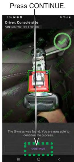
A green check mark will be displayed in the top right of the screen when the application is able to verify the repair.
