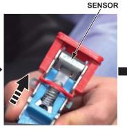
Insert the forks of the tool under the button bridge and slide it upward into place.
