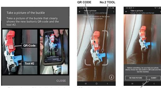
Take a picture of the buckle that clearly shows QR code on the new button, and the #2 tool inserted under the buckle bridge.
