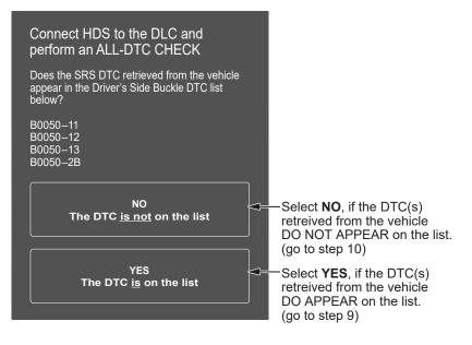
9. When **YES** is selected in the previous step, the application will direct you to do troubleshooting to identify the cause of the DTC. DO NOT MAKE A SELECTION UNTIL TROUBLESHOOTING IS DONE. There are several possible causes for the front seat belt buckle DTC. Refer to the service information for the DTC(s) retrieved from the vehicle.
