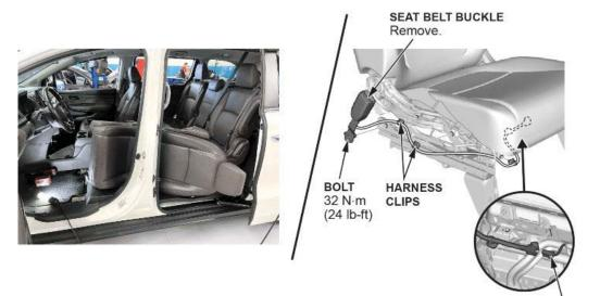
• Detach the harness clip(s), and connector clip(s).
