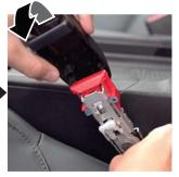
Then remove the upper cover by pulling it away and upward.
