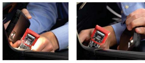
NOTE: Examples of buckles with residue that would cause the buckles to fail the residue check.
