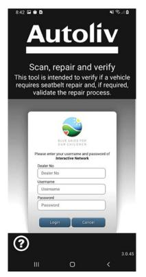
3. Scan the VIN to determine the buckle repair status.
