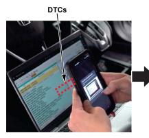
Connect HDS to the vehicle, perform an ALL DTC Check and expand the SRS/SWS DTC Menu to display the SRS DTC(s). DTCs VIN
