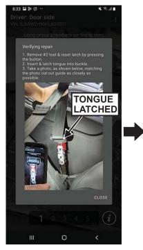
Insert the Seat Belt Tongue into the buckle and confirm it is latched. Pull up on the seat belt to provide a clear view of the buckle.
