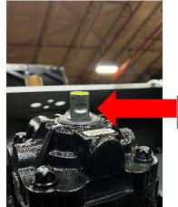
Align bolt with groove
