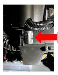
Align bolt with groove
