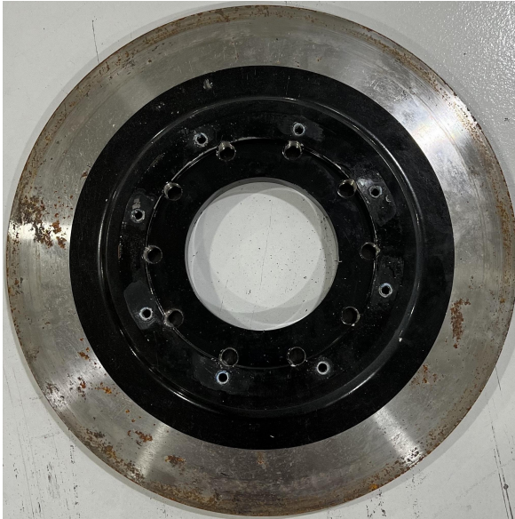
Figure 1 - Painted Rotor (Incorrect)
