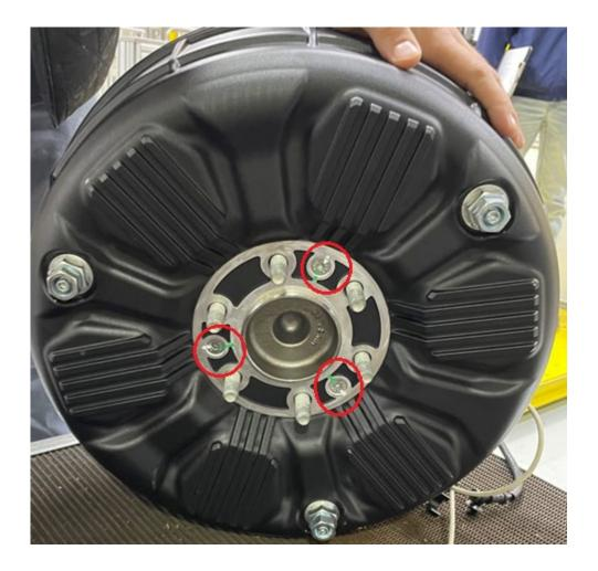
• Remove the 8bolts securing the rear knuckle to motor stator.
