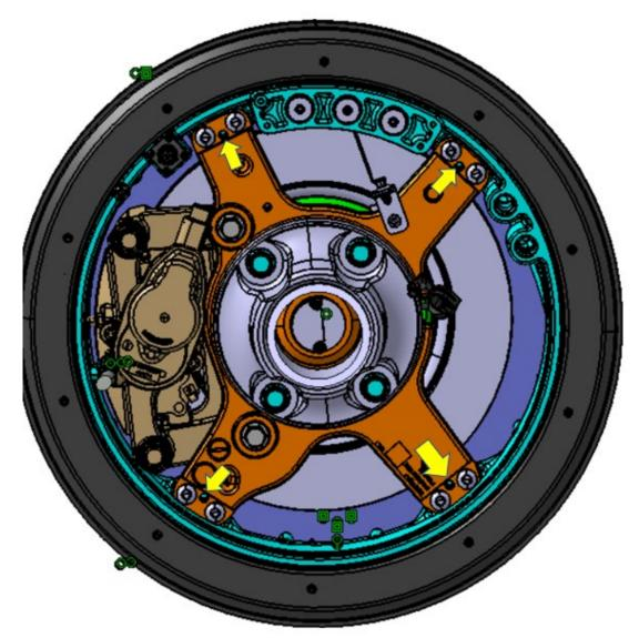
• Remove the caliper bolts and slide out the brake caliper.
