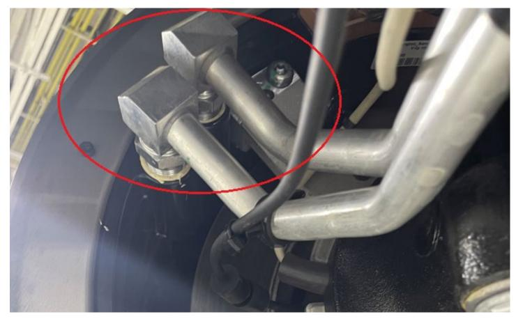
• Remove the Dust covers on the motor. Align the holes on motor rotor and motor stator to install the Brake service tools (BST).
