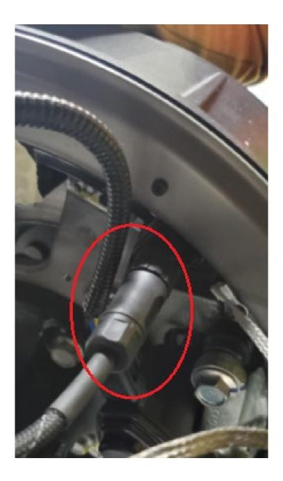
• Disconnect the brake jounce hose to brake line. Place a dripping pan to avoid any spills of brake fluid on the floor.
