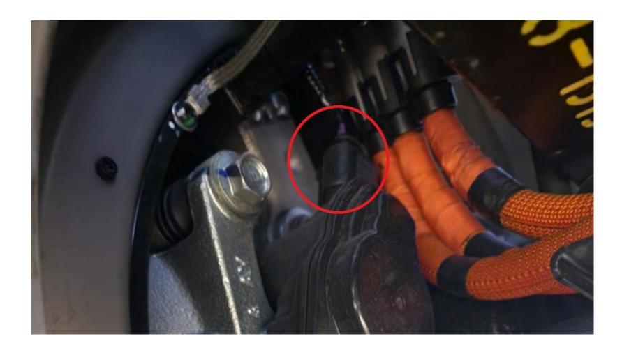
• Insert a blunt-ended bar ("pedal prop") between driver's seat and brake pedal, and adjust driver's seat position such that the brake pedal is pushed 1" to 2" from it's normal home position (this will greatly reduce the amount of brake fluid lost when the rear brake hoses are disconnected).
