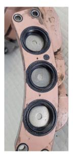
Make sure o-ring channels are clear and metal mushroomhead connections are clean of all contaminates.
